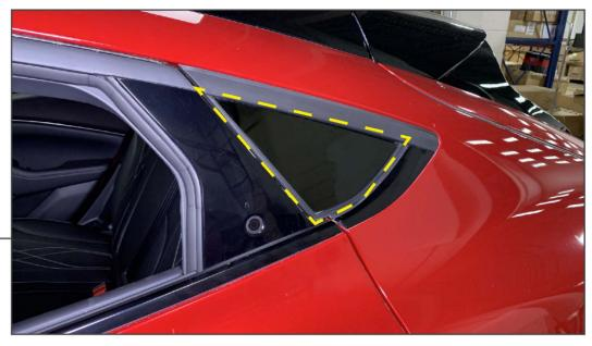
Clean the vehicle quarter window louver using the included adhesion promoter pads, allow to fully dry. Familiarize the window louver to the vehicle prior to removing the red tape backing.
