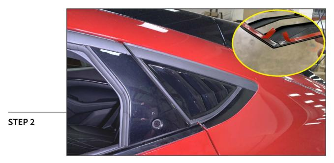
Once familiar with fitment on the vehicle, peel the red tape backing from the double sided tape. Align and apply the louver to the vehicle. Apply firm pressure to ensure proper adhesion.
