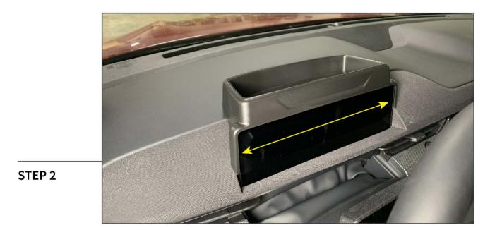
Place the sides of the tray around the sides of the screen, and slide down until the tray meets the dashboard.
