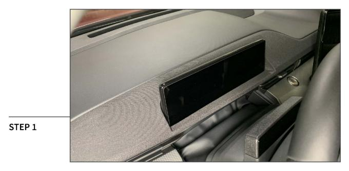
Clean the area around the driver screen using interior detailer and a microfiber cloth.
