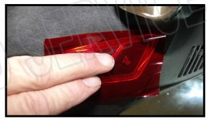
Start in the middle of the lens and work the film out toward the edges making sure to eliminate bubbles and wrinkles. It helps to lift the film with one hand and press the film outward with the other . You can use a credit card as a squeegee to press out any bubbles or creases.
