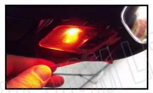
One extra sheet is provided in case you make mistakes. Remove the adhesive backing by placing a piece of scotch tape on each side then pull off the backing with the tape. Carefully lay the film over the light making sure the entire light is covered.
