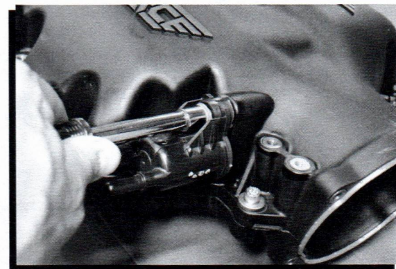
Figure 9 Install the EVAP Solenoid.
