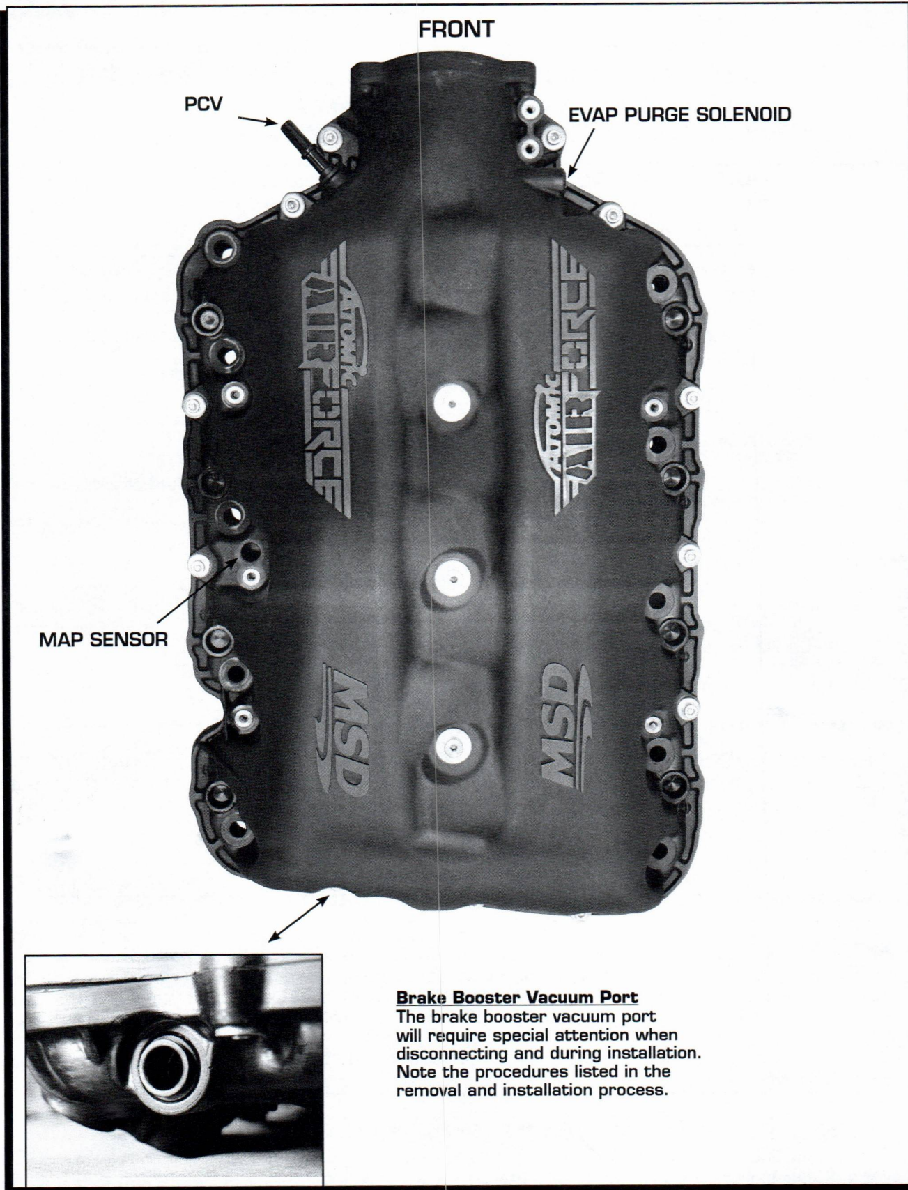
Figure 1 Vacuum Ports of the AirForce LT1 Manifold.
