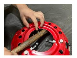
Fig 3 shows lever blocks being removed and the handle letting the lever up. Do this to all three levers and put them in your toolbox or discard them in the trash if you never intend to use them again. Again <u>CAUTION!!!</u> Should be taken not to place your fingers between the lever and the stamped steel cover at any time during this exercise. The handle could slip and catch your finger between the lever and cover incurring injury to or others.
