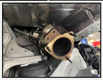
17. Now that the factory catalytic converters are out of the car, swap over the gaskets and sensors to the new Fabspeed sport cats. It's also recommended to install the 2 long bolts on the left side cat before putting it in the vehicle. A small dab of grease can help hold the header/cat flange gaskets in place during installation.
