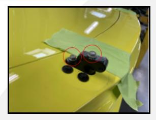
5. Reaching through the wheel wells, remove the 3 fasteners connecting the bumper to the body on each side.
