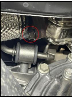
10. Return back to the cargo area and remove the remaining 4 flange nuts.
