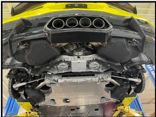
4. Before the bumper can be taken off, the wing must be removed first. YOU MUST HAVE A 5 POINT TAMPER-PROOF T30 BIT. Once the wing is off, undo the 2 long 10mm bolts on each side.
