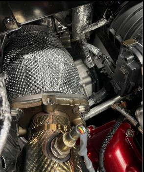
18. Once the sport cats are in the vehicle, reinstall the factory heat shielding and begin reassembly of the vehicle. Again, a valve relearn may be required to regain full function of the valves. Once the muffler is reinstalled, be sure to start the vehicle and check for leaks before fully reassembling everything. Some smoke/burning is normal upon initial start up. Afterwards, get out on the road and enjoy your new Fabspeed products!
