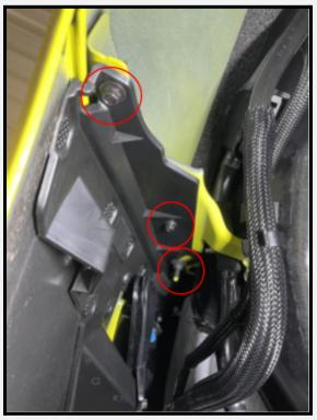
6. The next step is to remove all of the T15 fasteners along the upper lip of the bumper. There are 2 that can be easy to miss, located farthest to the left and to the right.
