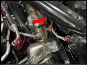
13. Unplug both secondary oxygen sensors, as they will come out with the factory converters.
