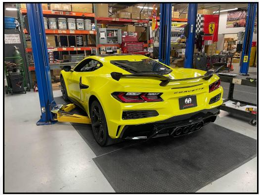
2. Begin disassembly by removing rear wheels and wheel well liners. There is an assortment of push-pins, T15, and 7mm fasteners. One of the T15s is hidden behind the mudflap.
