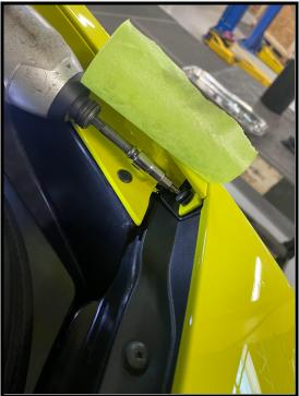
7. Now to pull the bumper off the vehicle. Be very careful while doing so, as there are shims included from the factory under the bumper itself. Take note of the quantity and position of these shims to assume proper panel gap upon reassembly. Additionally, there are 3 connectors that will have to be unplugged once the bumper is partially removed.
