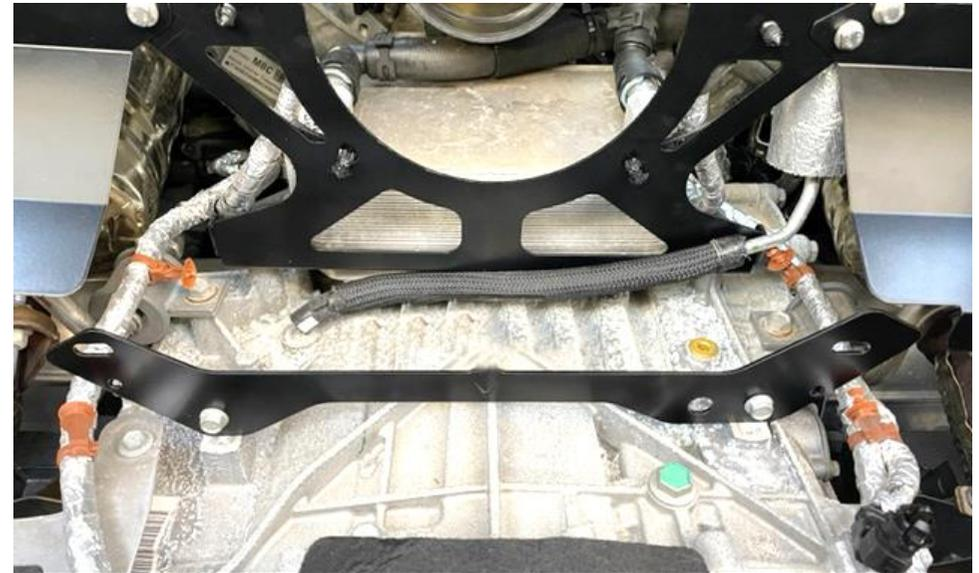
45. Using the stock screws removed previously for the airbox, secure the brace on the remaining mounting points for the airbox as shown.
