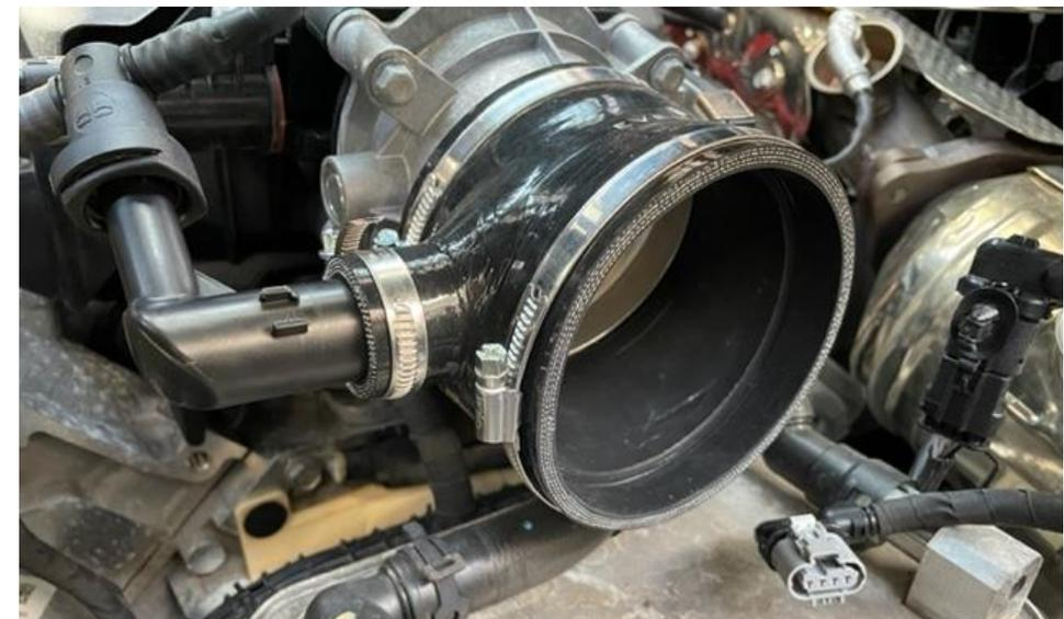
19b. Install the silicon hose onto the throttle body and push the breather elbow into the clip again. It will click into place. Make sure the silicon is fully pushed onto the throttle body. It should be flush on the inside all around. Now secure the clamp around the throttle body and the breather.
