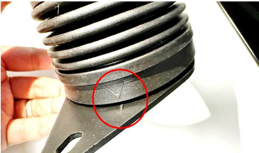
32. Push the provided flexible hoses onto the inlets. Line up the V logo on the hose to the mark on the inlet as shown. Clamps are not required. Make sure the hose is pushed down evenly all around. **The Top of the hose has "C8 Filter Side" marking on it.**
