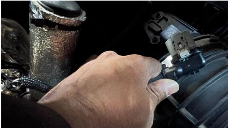
11. Unclip the MAF sensor plug from the back of the airbox.
