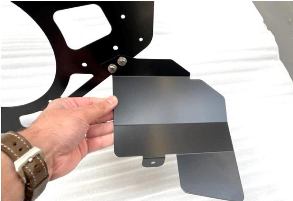
36. Secure the shields to the frame using the holes shown.
