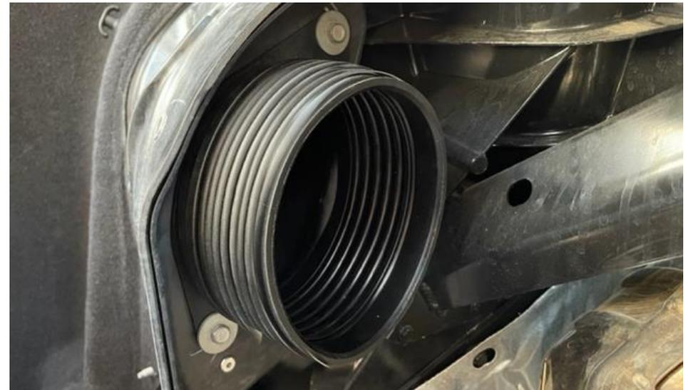
33. Take the Left side inlet and flexible hose and secure it to the left cold air feed using the stock screws removed previously. Repeat for the right side.
