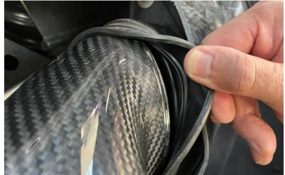
51. Pull the flexible hoses over the intake on both sides. Ensure the hoses are fully latched onto the carbon. No clamps are required.
