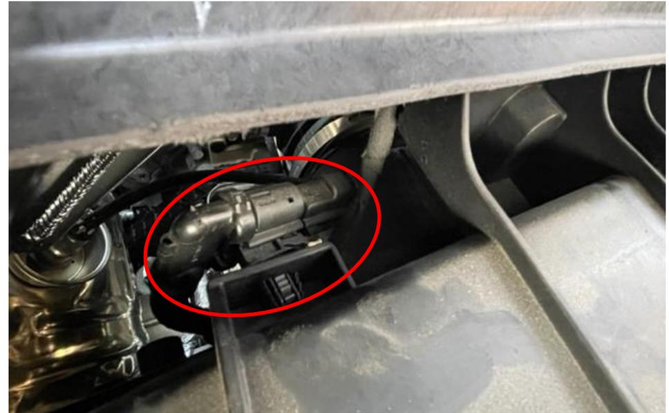
10. At the top of the airbox there are also a couple of plugs which need to be removed on each side.
