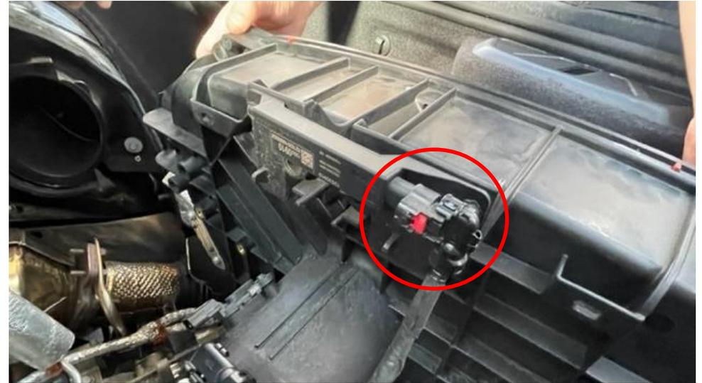
14. Disconnect the plug from the sensor at the top of the airbox.
