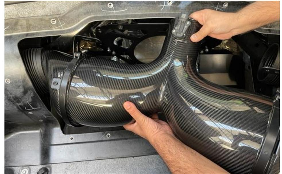
48. Push the intake into one flexible hose and move it into place through the frame and into the silicon hose on the throttle body.
