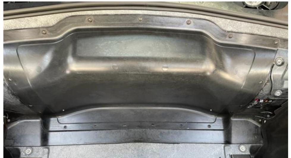
2. Now remove the screws holding the trunk panel in place. We will re-use these screws for the new panel.
