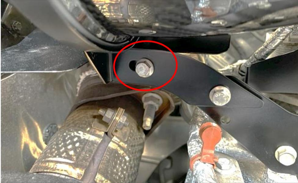
58. Take another M6 screw and nut. Secure the bottom of each shield to the lower intake bracket as shown.
