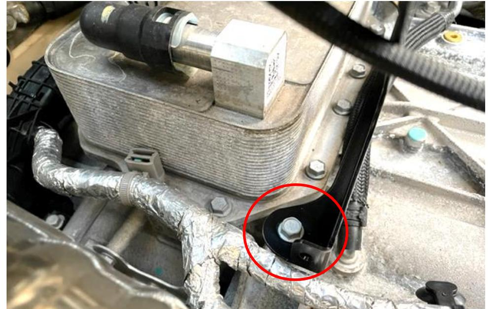
39. Use the stock screws previously removed to mount the frame as shown on both side.
