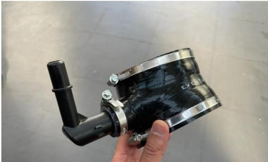
19. Take the new silicon hose and insert the plastic breather elbow into the side opening. Push it in as far as possible. Leave the hose clamps loose for now.
