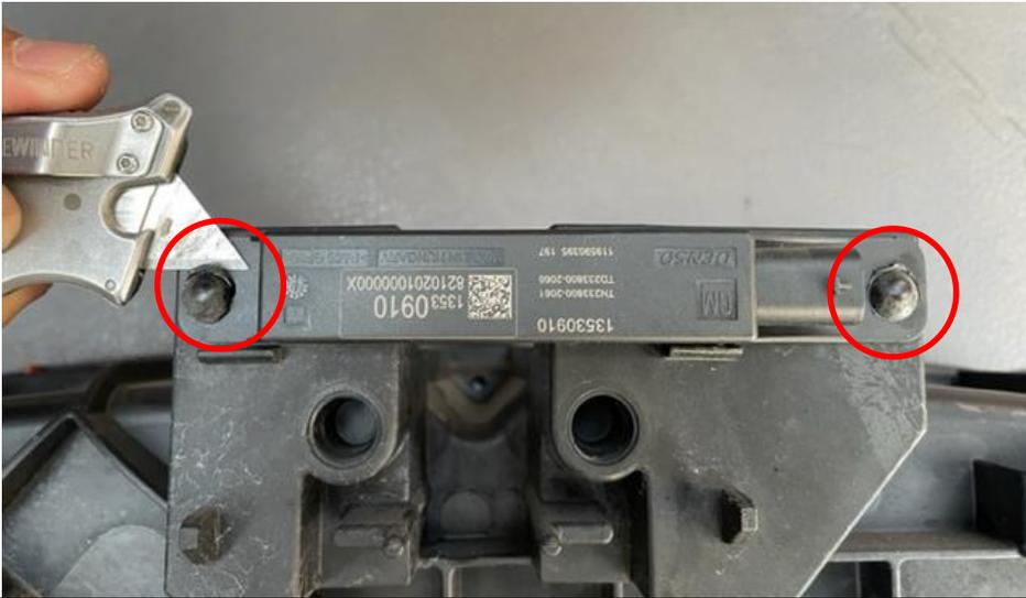
17. Using a sharp knife – carefully cut the plastic rivets holding the antenna to the top of the airbox. Remove the antenna from the airbox.
