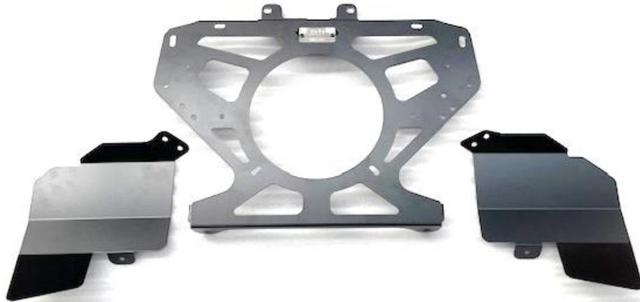
34. Take the 2 shields and the middle frame as shown. Lay the shields as shown on the left and the right. They are handed.
