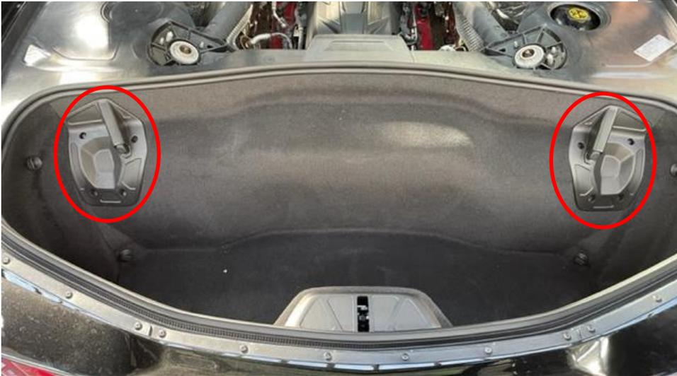
1. Start by removing the rear carpet. This can be done by removing the roof mounts on each side and the plastic clips holding the carpet down.
