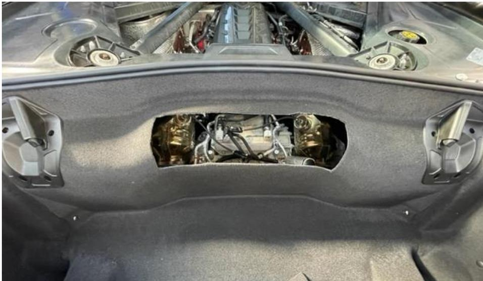
22. Using a sharp utility knife, make an access hole in the middle of the carpet. This will allow you to mark the inside.
