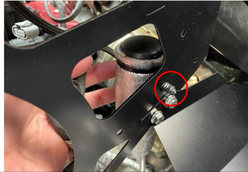
41. Clip the insulated module into place behind the frame.
