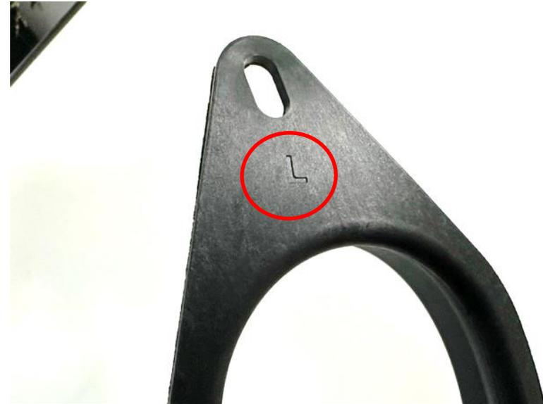
31. Marking shown on the base to indicate this is a Left side inlet. Looking at the engine from the back of the car, the L inlet goes onto the left side and the R inlet to the right side.
