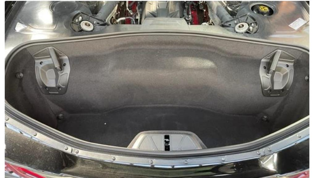
21. Before installing the intake – we will now cut the carpet for the new clear panel. Put just the carpet back into place and secure with the 2 roof mounts on each side.
