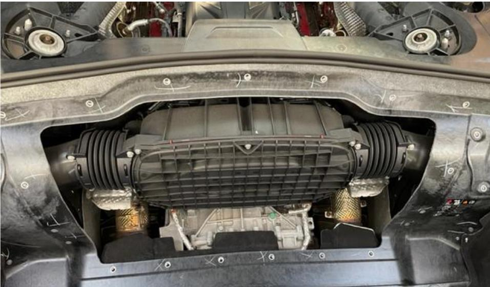
3. With the panel removed we can now start to remove the airbox.
