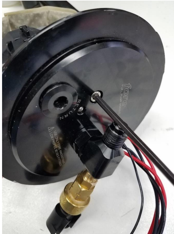
Photo 3. Remove the single screw from the top of the module hat. Support the mid-span platform by hand so it does not fall off.
