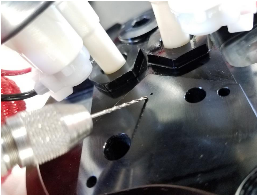
Photo 5. Using the drill bits provided, drill out the hole as shown. For TI450 pumps, use the 0.041" bit. For TI525 pumps, use the 0.051" bit. Only increase the size of this hole, do not drill past the manifold passage and into the hat. A pin vise works well to hold the drill bit. BE SURE TO USE THE BIT TO CLEAR THE HOLE OF BURRS AND CHIPS.
