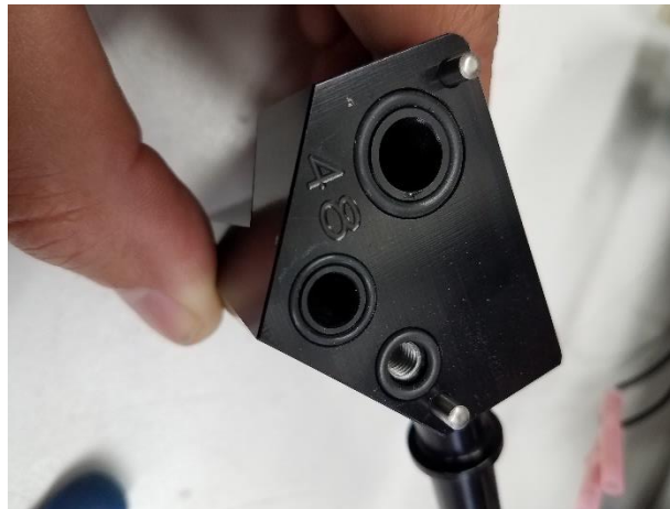
Photo 6. Confirm that all of the o-rings and dowel pins are in place and seated correctly. Some versions may appear a bit different, but the premise is the same.
