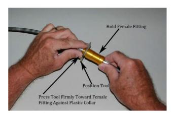
Assembly is easy, just press the two fittings together. Separation is just as easy, position the separation tool onto the male fitting between the plastic collar and the raised shoulder near the AN-4 hose. Press the separation tool towards the female fitting until the fittings separate. No fluid leakage will occur.
