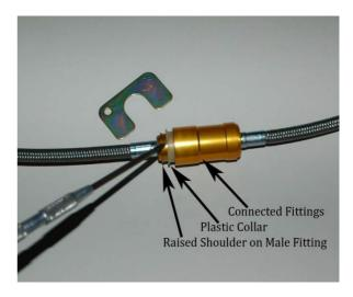
The above photos call out the key components including the male and female fittings, separation tool and plastic collar. Do not remove the plastic collar from the male fitting!
