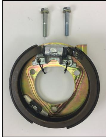
2. Your new park brake assembly comes with bolts for the cable bracket. It has zip ties holding the actuator & cable bracket in place. Cut these and set the cable bracket aside.
