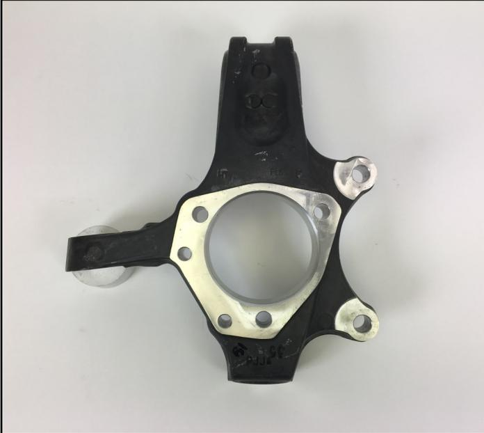
1. This installation begins at the point at which the bare knuckle has no components installed. (Passenger side rear shown)
