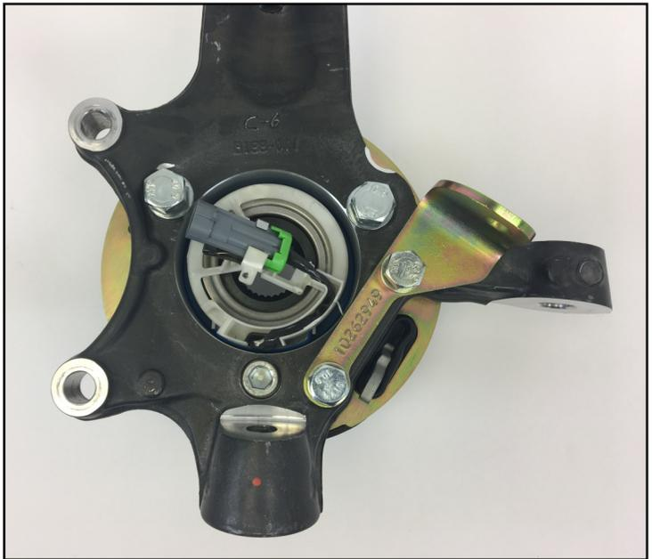
5. Place the hub with the park brake assembly on the knuckle, making sure to align the hub bolt holes, park brake assembly holes, and actuator / cable bracket holes.
