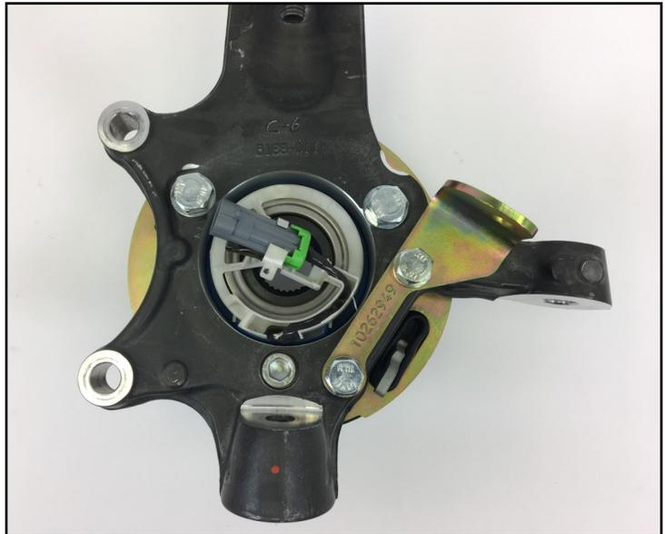
7. Outboard view of the park brake assembly installed. (Passenger side rear shown)
