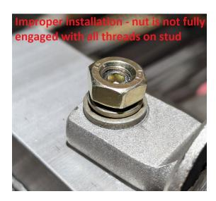
Nut installed ABOVE the turned portion of the end of the stud. This will cause the end of the threads to rip out when torqued
