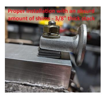
Stud installed with a large amount of shims, removing 1.5 degrees of camber. There should be no reason to use this number of shims, but we still have minimal protrusion of the stud.
