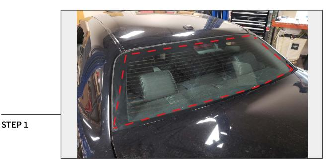
Begin by thoroughly cleaning the rear window glass using the supplied alcohol pad to ensure the glass is free of any and all road debris.
