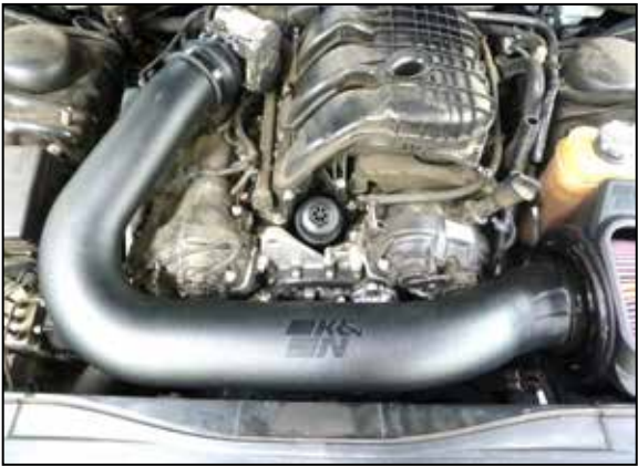
15. Install the K&N intake tube into the air filter and then into the coupler at the throttle body. Do not secure the hose clamps yet.
