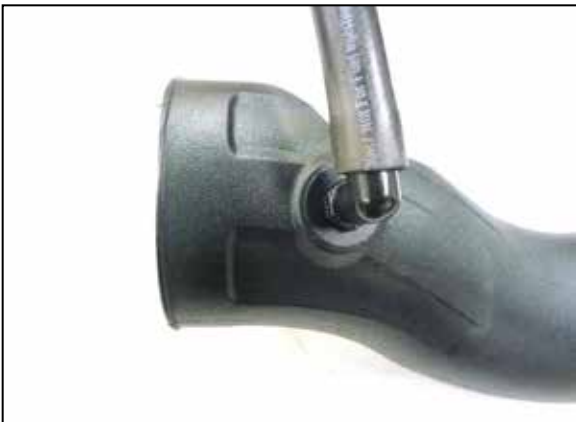
12. Install the provided CCV hose onto the 90-dgree CCV fitting for the early models.
