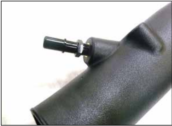
10. Partially place air filter into air box and Install the K&N air filter housing into the vehicle. NOTE: Before Install of the filter, tighten insert nut using 14mm socket. Now push K&N air filter into the K&N air filter housing. Secure with the factory mounting bolt.
