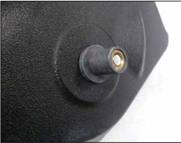
8. Install the provided insert nut onto the K&N filter housing using the provided hardware. This will seat into the inside fender hole of vehicle.
