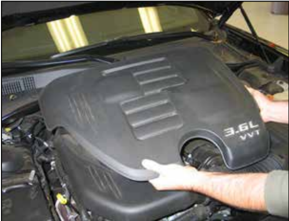
2. Lift the engine cover and remove it from the vehicle.
