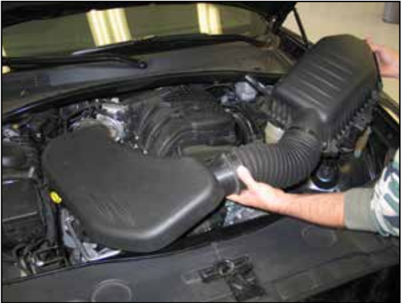
7. Remove the complete stock intake system from the vehicle.
