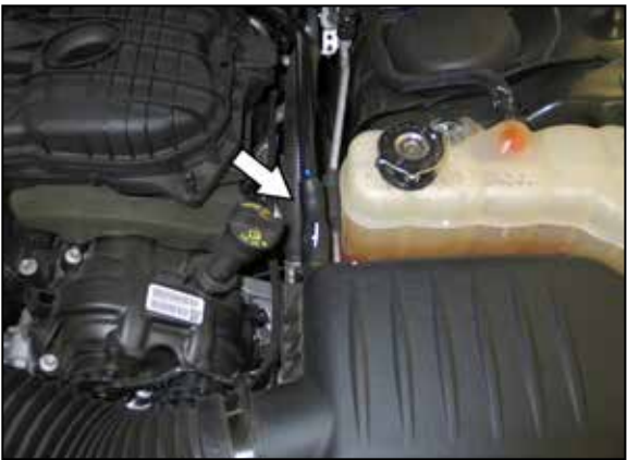
4. Disconnect the CCV hose from the air filter housing. NOTE: On later models the CCV line connection will be near the throttle body.
