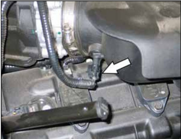
3. Disconnect the IAT sensor electrical connection.
