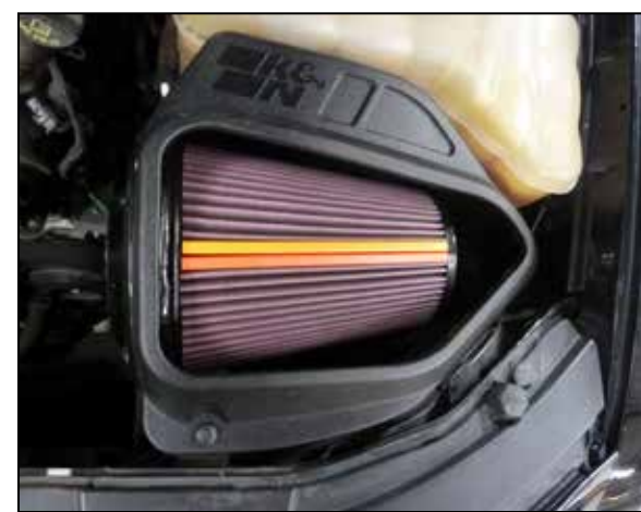
10. Partially place air filter into air box and Install the K&N air filter housing into the vehicle. NOTE: Before Install of the filter, tighten insert nut using 14mm socket. Now push K&N air filter into the K&N air filter housing. Secure with the factory mounting bolt.
