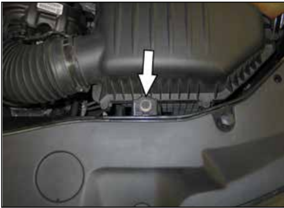
6. Remove the bolt that secures the air filter housing to the core support.
