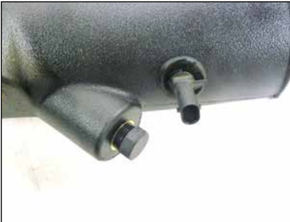
14. Remove the IAT sensor from the factory intake system, remove the O-ring from the sensor and then install it into the K&N intake tube using the provided grommet.
