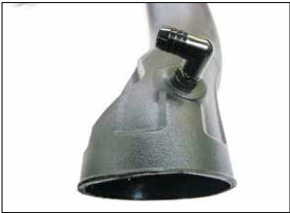
11. Install the provided quick connect fitting and npt plug into the K&N intake tube. 2011-19 models will use the 90-degree fitting near the filter end of the tube. 2020-23 models will use the straight fitting near the throttle body end of the tube
