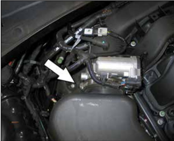
5. Loosen the hose clamp that secures the intake tube to the throttle body.
