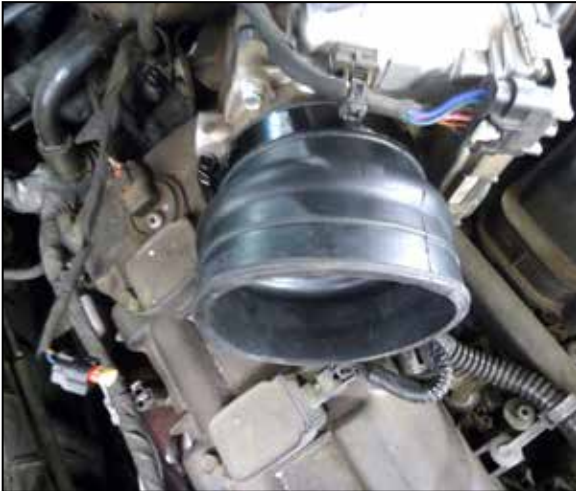
13. Install the provided hump coupler onto the throttle body and secure with the provided hose clamp.
