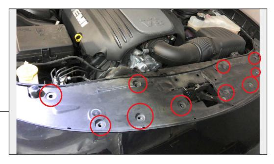
Using a jack and jack stands, support the vehicle off the ground. Using a panel removal tool, remove the (10) plastic push clips from the radiator cover. Remove the radiator cover from the vehicle.
