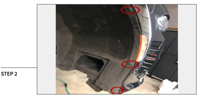
Remove (3) push clips from the fender liner behind the bumper. Repeat this procedure for the opposite side.
