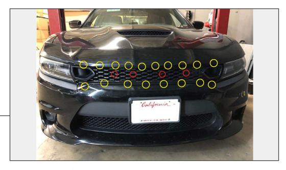
Using a panel removal tool, remove (4) push clips behind the grille, then remove the grille by manipulating the (18) plastic tabs surrounding the grille. Install the new grille in reverse order of removal.
