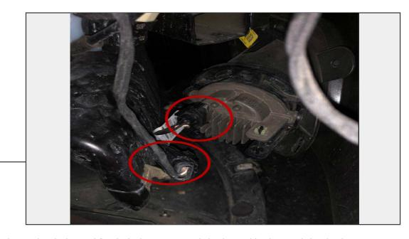
Unplug the side marker light and fog light harnesses. Slide the red locking tab back, then press down on the connector and slide the connector off the light. Repeat this procedure for the opposite side.
