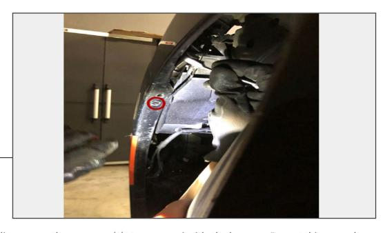
Pull the fender liner away, then remove (1) 7mm screw inside the bumper. Repeat this procedure for the opposite side.
