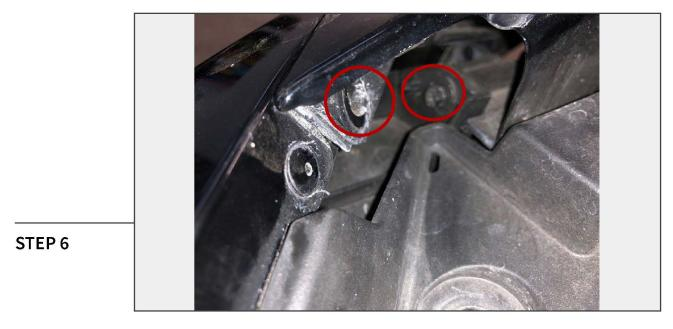
Remove (2) 10mm bolts from inside the bumper to release the bumper from the fender. Repeat this procedure for the opposite side.
