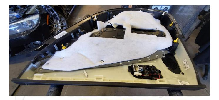
Remove the wire hold down by the front of the door and pull the harness tighter until you have an inch or so of extra slack at the front.
