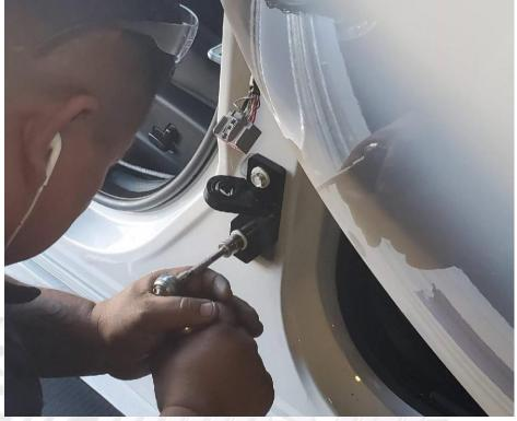
**19)** Install the shock. You must use Loctite on the threaded end of the shock. *Hint\** (You will need a helper to raise the door). (1) (Slip the spherical rod mount into the spherical ball bearing. Then screw the shock into the swivel shock end that is pre-installed on the hinge. After the shock is installed secure it by installing the pin in the bottom shock end by tapping it in with a hammer (2)
