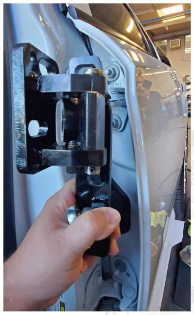
6) You will need to cut off the bottom stud on the top door hinge, then drill and tap 1 hole on each side in the door to complete the install.
