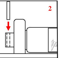
Tip: Smear grease around the spherical shock bearing before installing the shock.
