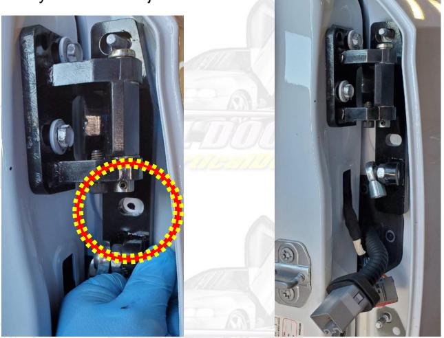
**14)** After marking for the hole, remove the door with a helper and place it back on the stand. You will then drill and tap a new threaded hole where the mark you just made is. The thread size is M8 x 1.25
