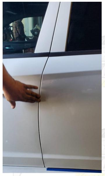
**17)** Open the front door and prepare to open the rear door. Carefully open and support the weight of the door because it will probably drop when opening. Then you can adjust the adjustment bolt like in step 10 so that the door lines up perfectly with the latch when closing.
