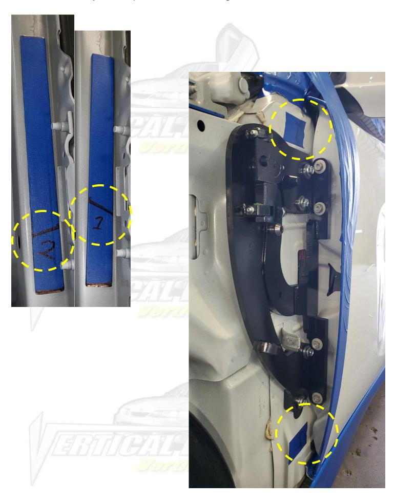
11) Remove original door hinges and Install the New Vertical Doors Inc. System. You will use the OEM Nuts on the door side. Use the bolts and heavy-duty washers provided on the chassis side.
