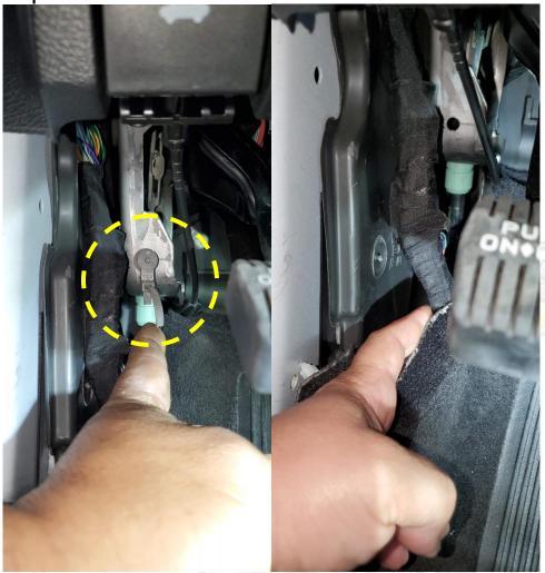
4) Unplug the door harness from the chassis. Un-clip the portion of the harness secured to the chassis so that you can pull the connector to the outside.
