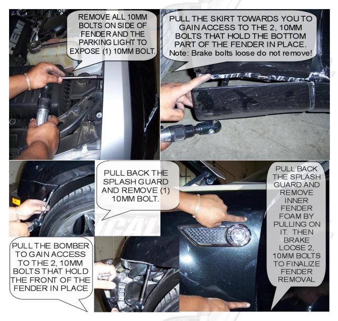
To remove the fender, lift up the top of the fender toward you and then slip out the bottom end.
