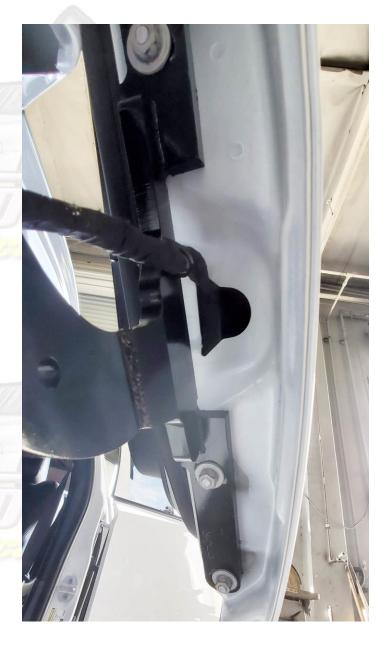
8) You will need to remove the door panel as well. You will insert the chassis portion of the harness through the hole you made in the end of the door. Plug the two connectors together inside the end of the door and secure out of the way of the window etc. with zip ties
