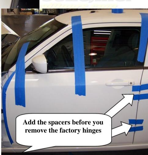
Before removing the factory hinges you MUST mark the factory location of the door on the vertical and horizontal planes. Also mark and measure the distance between the apron and the edge of the door by the top and bottom hinge.
