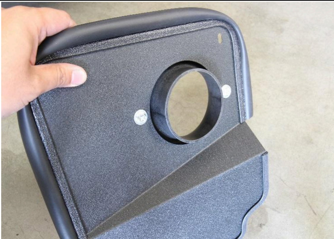
15. Install the velocity stack onto the heat shield as shown with 2 bolts and washers.
