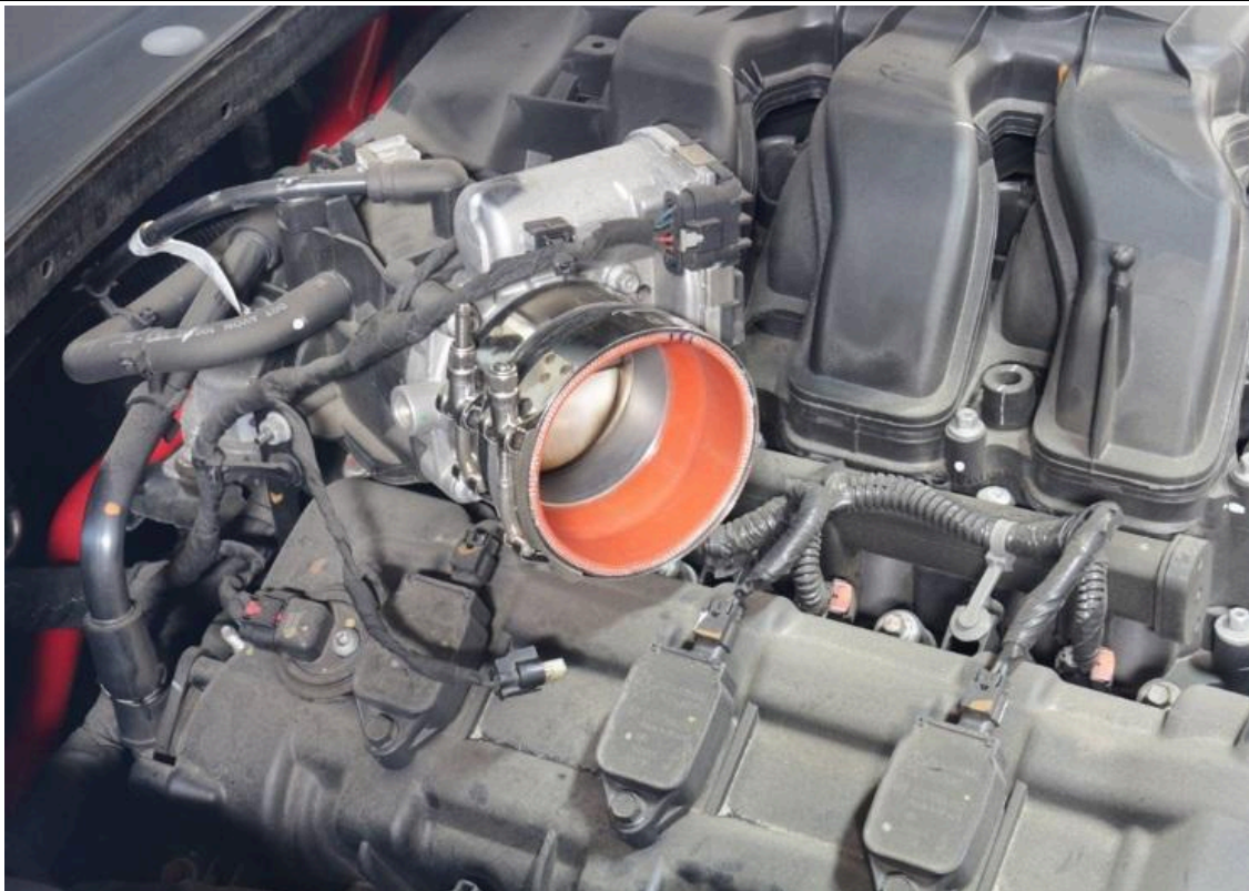
8. Install the reducer coupler with their corresponding T-bolt clamps onto the throttle body.
