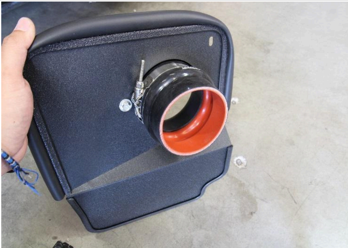
16. Install the last hump coupler onto the velocity stack with its corresponding T-bolt clamp.
