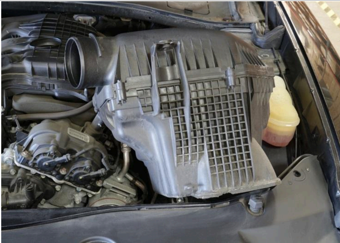
7. Remove the factory air cleaner assembly from the engine bay.
