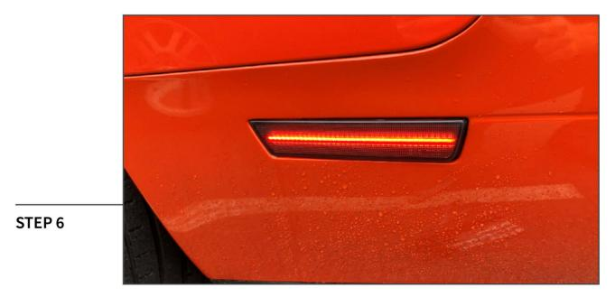
Install the LED side marker light into the bumper. Firmly press the light into the bumper to ensure the light is correctly seated.
