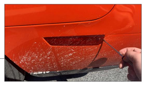
Using a flathead screwdriver, gently pry the side marker lens from the rear bumper.
