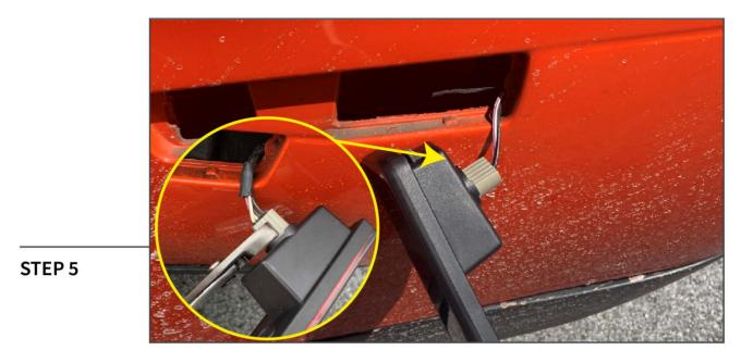
Install the light socket into the LED side marker housing by twisting the light socket clockwise.
