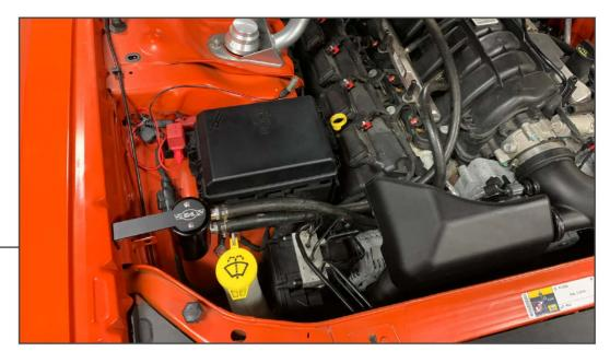
Route the supplied vacuum line from the oil separator to the intake manifold. \*\*If you plan on reinstalling the engine cover, make sure the vacuum lines clear. Test fit the cover before cutting the lines. The top port on the oil separator will connect to the front port on the intake manifold. The bottom port of the catch can will connect to the rear port on the intake manifold.
