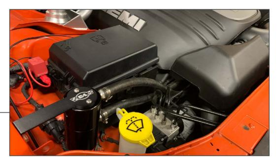
Reinstall the engine cover. Installation is now complete. Empty the catch can as needed.
