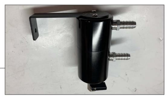
Install the supplied bracket to the oil separator using (2) M4x0.7 machine screws, (2) M4 flat washers. Install the ball valve on the bottom of the oil separator, use thread sealant to ensure a leak free installation.
