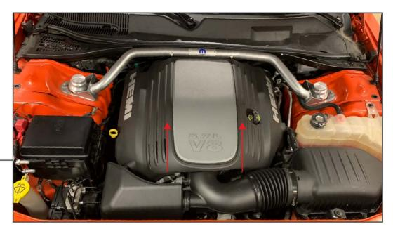
Pull up on the engine cover to release it from its retaining posts.
