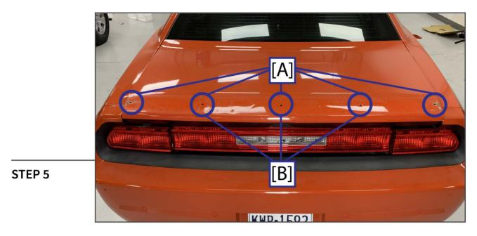
Drill (5) pilot holes using a 1/8" drill bit [A].
