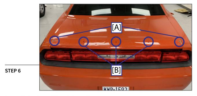
Using a 5/16" drill bit, drill holes indicated [A].
