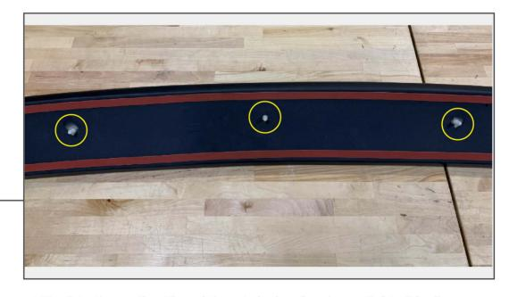
Install (3) Alignment Pins into the spoiler. Thread them in by hand and snug tight with pliers.
