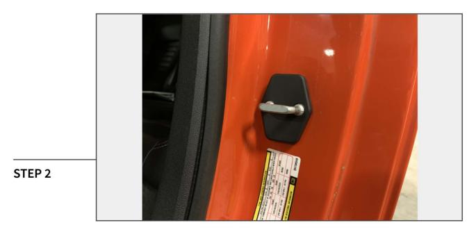
Align the striker cover to the vehicle hinge. Press on until fully seated.
