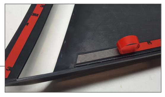
Remove the tape backing, align the louver to the window and press it on.
