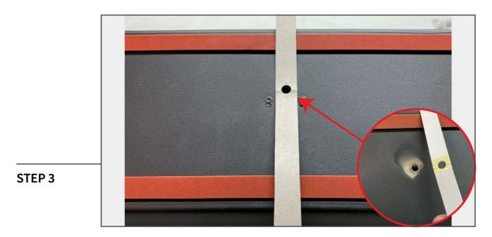
Adhere the provided (5) Alignment Strips to the spoiler. Peel the adhesive backing off the middle of the strip, then align the hole in the strip with the hole in the spoiler.
