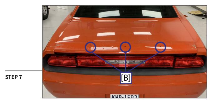
Insert (3) Plastic Grommets into the drilled holes indicated [B]
