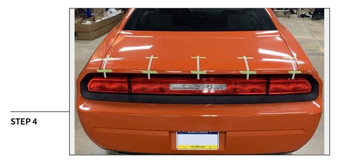
Align the middle strip with the trunk release button on the spoiler. Using masking tape, adhere the (5) alignment strips to the trunk lid to secure them in place. Lift the spoiler away from the vehicle.
