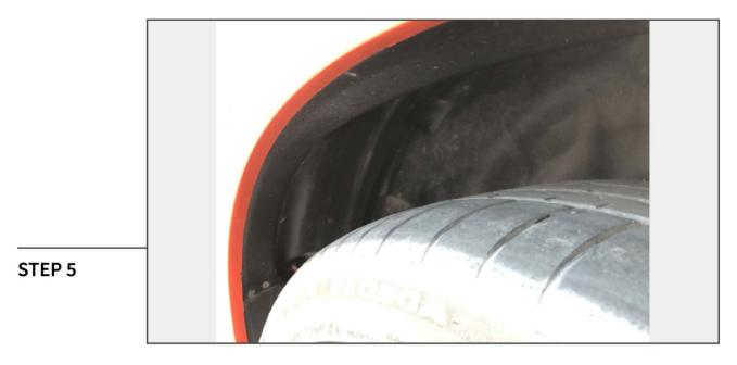
Install the fender liner extensions using the provided screws.
