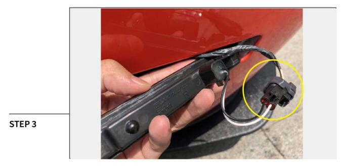
Connect the LED marker light to the factory wiring harness.
