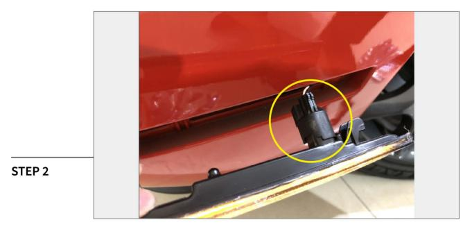
Depress the clip on the wiring connection and remove it from the factory light.
