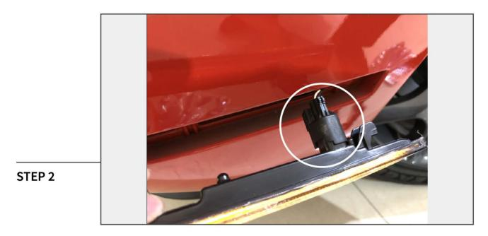
Depress the clip on the wiring connection to remove it from the factory light.
