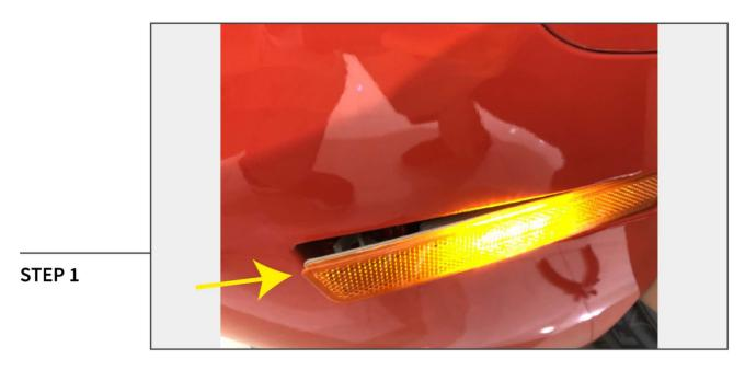
Using a thin non marring pry tool, depress the clip at the front of the marker light to remove it from the bumper. If you do not have non marring tools, you can reach behind the bumper to depress the clip.
