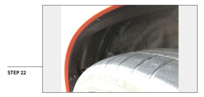
Install the fender liner extensions using the provided screws.
