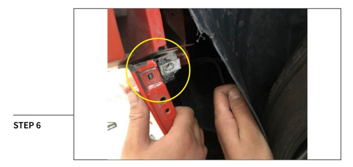
Peel back the fender liner to access the (1) 10mm bolt.
