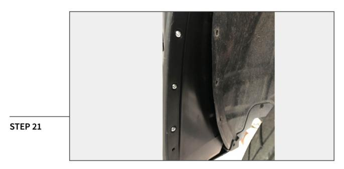
Install the splash shield extensions using the provided screws.
