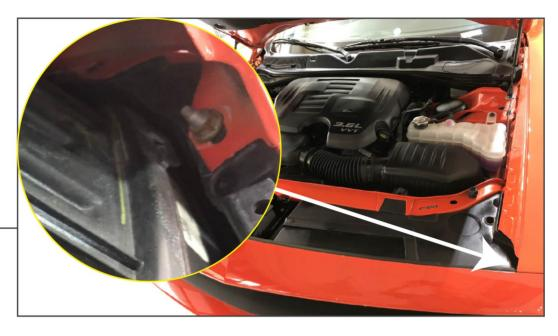
Using a 10mm wrench, locate and remove the 10mm nut that secures the bumper to the fender just behind the headlight.
