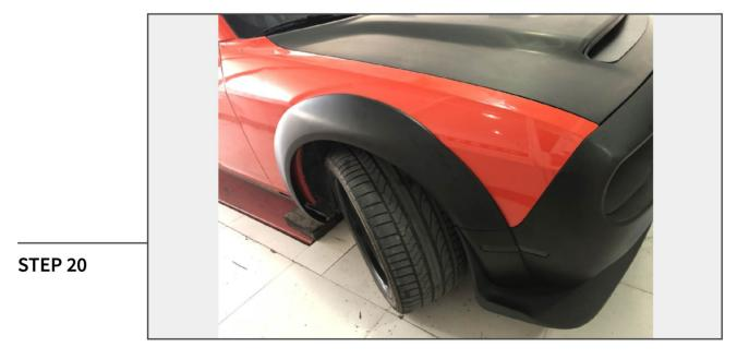
Align the clips with the holes drilled in Step 1. Firmly press the flares onto the vehicle. Apply firm even pressure over the tape mounting locations to ensure proper adhesion.
