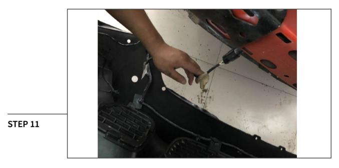
With a helper, reconnect the wiring harness and place the bumper cover on the vehicle.
