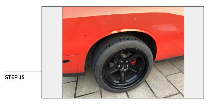
Using a 5/16" drill bit and drill, careful drill the locations marked in Step 2.
