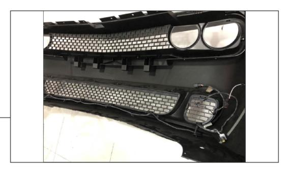
Using a panel removal tool, remove the harness from the factory bumper and transfer it to the new bumper cover.
