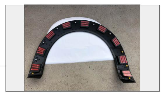
Install the supplied 3M double sided tape as shown above. \*\*Note: Ambient air temperature needs to be above 50\*F for proper tape adhesion.
