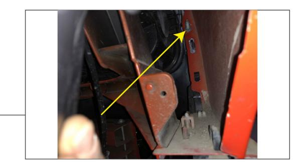
Peel back the fender liner to access the (1) 10mm bolt.
