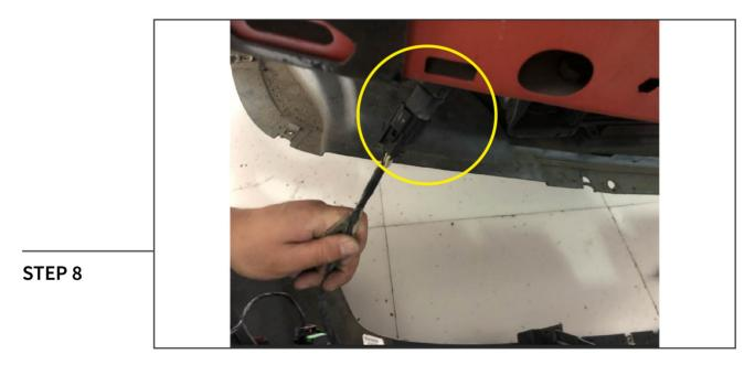
With a helper, carefully remove the bumper from the vehicle. Unplug the wiring harness from the bumper.
