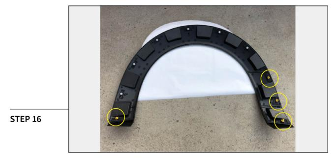
Install the supplied clips onto the fender flares. Note the locations that require the yellow clips circled above. Use white clips in all other locations.
