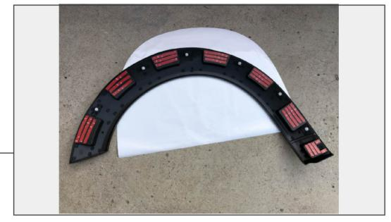
Follow the same process to clean the front fenders as you did the rear. Align the template to the vehicle and drill the 5/16" holes. Install the clips and tape to the fender flares.
