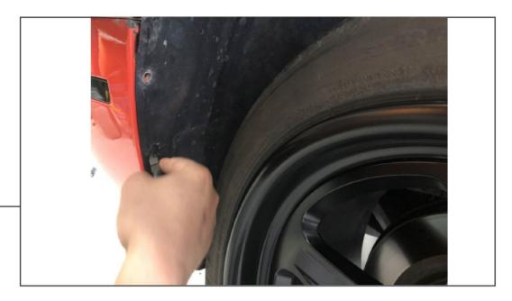
Using the trim panel removal tool, remove the (3) push clips securing the fender liner to the bumper.
