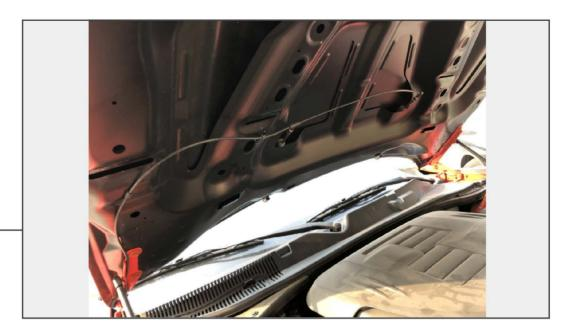
With a helper, reinstall the hood using the factory bolts. Loosen the mounting bolts and adjust the hood front-to-back and side-to-side for best fit. Slowly close the hood and adjust as needed. Then, reinstall the windshield washer hoses and nozzles.
