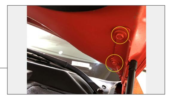
With a helper, remove the (2) 13mm nuts on each hood hinge. Then carefully remove the hood from the vehicle.
