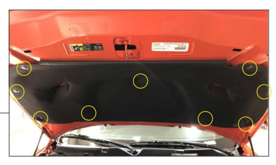
Begin by raising the hood to access to the under hood insulation. Using a trim panel removal tool, carefully remove the (9) Push clips securing the insulation to the underside of the hood.
