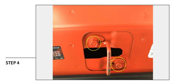
Using a 10mm socket, remove the (2) bolts securing the hood latch to the hood.
