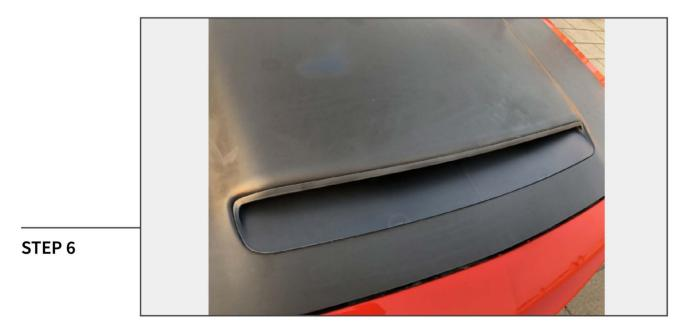
Install the hood insert by firmly pressing it into place. The insert will snap/clip into the hood.
