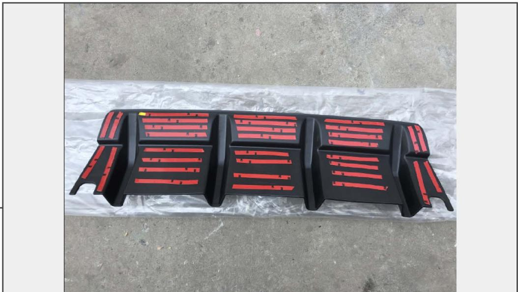
Apply the supplied tape to the rear of the diffuse as shown. Test fit the part prior to peeling off the tape backing. Once you are comfortable with how the part fits, peel off the tape back.
