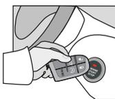
Place the OEM remote (no battery) close to the front of START/STOP button exactly as shown.
