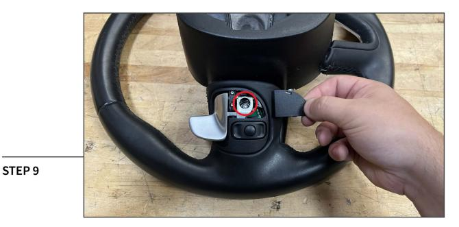
Turn the steering wheel face down on a workable surface. Use a small pry tool to remove the rear steering wheel control panel cover. Remove (1) T-20 Torx screw from the steering wheel control panel.
