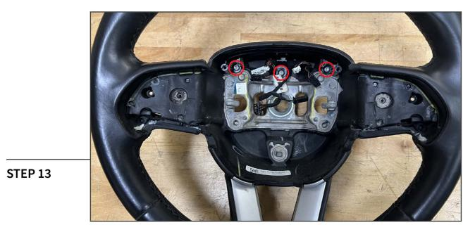
Remove (3) T-20 Torx screws from the steering wheel trim panel, and remove the trim panel and wiring harness from the steering wheel.
