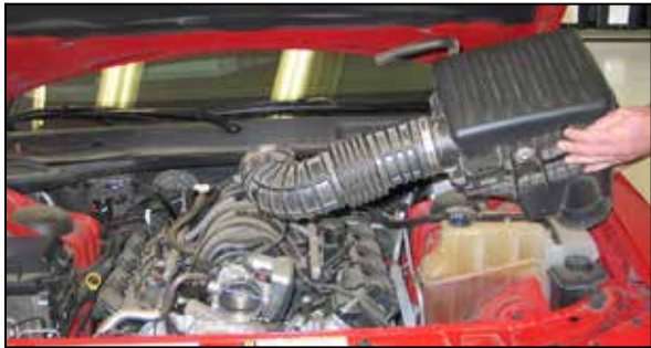
8. Lift and remove the complete intake assembly from the vehicle. NOTE: K&N Engineering, Inc., recommends that customers do not discard factory air intake.
