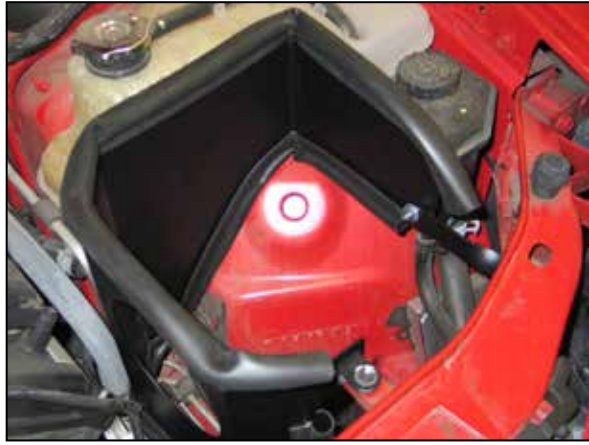
12. Install the heat shield assembly into the vehicle and secure to the bracket installed in step #9. Then secure the "L" bracket with the factory bolt removed in step #6 to the airbox mounting location.
