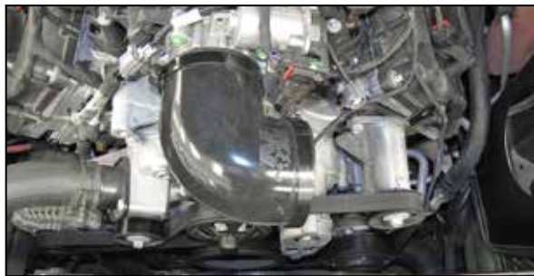
14. Install the silicone hose (084088) onto the throttle body and secure with the provided hose clamp.
