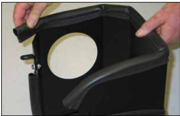
11. Install the two pieces of edge trim onto the heat shield as shown; be sure to leave a gap at the bracket mounting locations.
