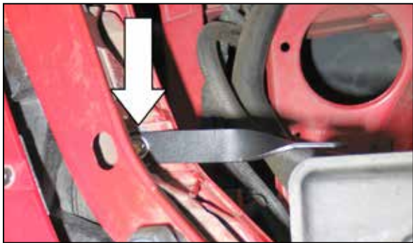
9. Install the twist bracket (070772) onto the core support using the provided hardware through the existing hole as shown. NOTE: On vehicles equipped with HID headlights, the bracket mounting bolt will need to be installed from the bottom up. This may be difficult but it will fit.
