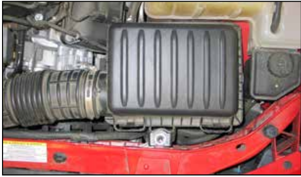
7. Loosen and remove the airbox mounting nut shown.
