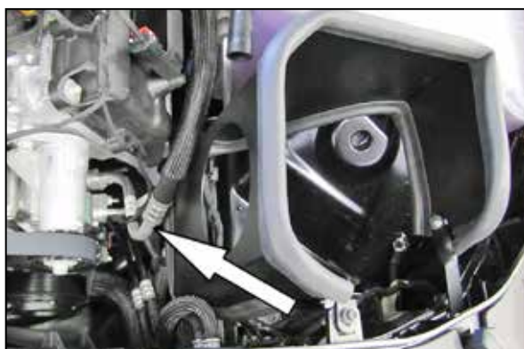
12a. Due to vehicle manufacturing tolerances, the A/C lines on some vehicles may need to be repositioned slightly so that they do not contact the heat shield. To adjust, grab the A/C line on the aluminum section and carefully apply pressure in the desired direction until clearance is obtained.
