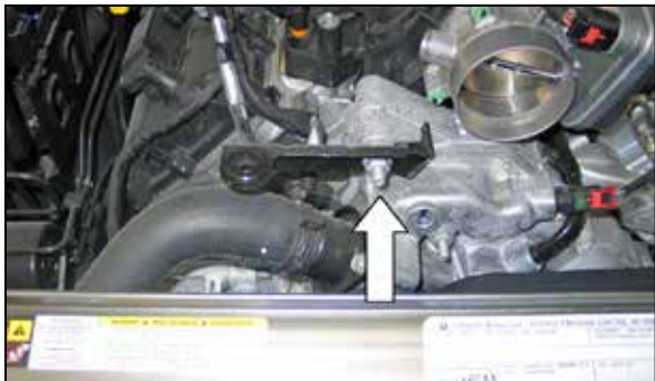
8a. On vehicles equipped with an intake resonator, remove the nut shown which secures the resonator bracket and then remove the resonator bracket from the engine.
