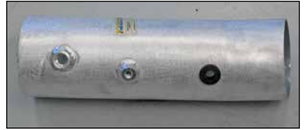
16. Install the provided grommet into the K&N® intake tube as shown.
