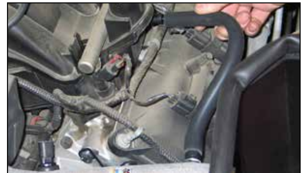
20. Install the provided crankcase vent hose onto the vent port on the valve cover and then connect the open end to the fitting installed into the K&N® intake tube. Some trimming of the crankcase vent hose may be necessary.
