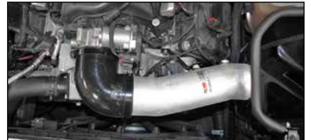
19. Install the K&N® intake tube into the silicone hose at the throttle body and align with the heat shield and mounting bracket. Secure the intake tube with the hose clamp and hardware provided.
