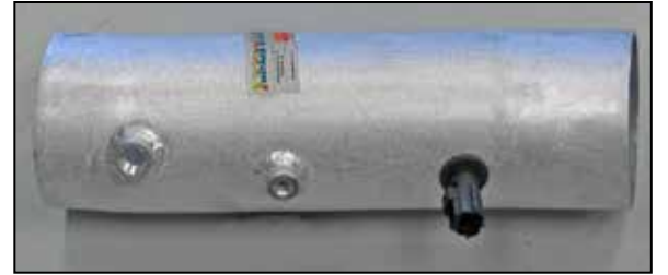
17. Install the inlet air temperature sensor into the grommet installed in the previous step.
