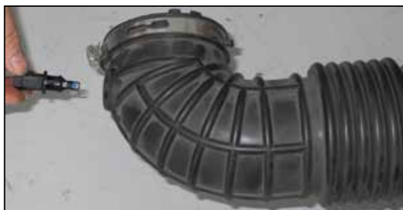
15. Remove the inlet air temperature sensor from the stock intake hose as shown. NOTE: Be very careful when handling the inlet air temperature sensor as it is very fragile. NOTE: The inlet air temperature sensor may be a different style than the one shown.
