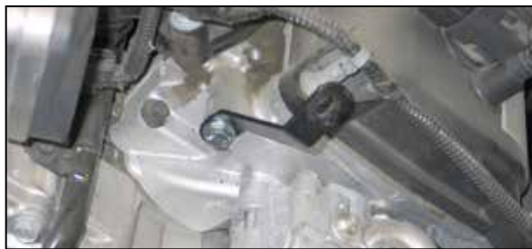
13. Using the provided hardware, install the tube mounting bracket (010088) onto the engine as shown. The 1/8" thick spacer (08129) should be placed between the bracket and engine.
