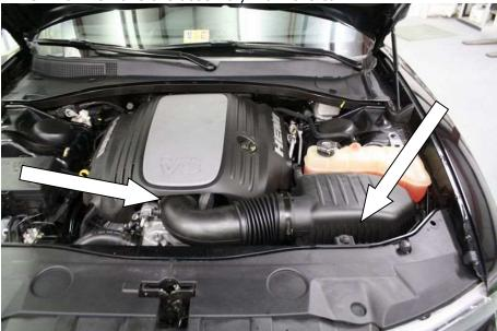
4 Remove the rubber location grommet from the stock air box and install into the hole in the apron.
