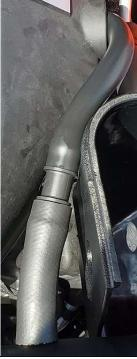
8 Rotate the tube so the filter is low in the shield and **HAND** tighten all clamps.
