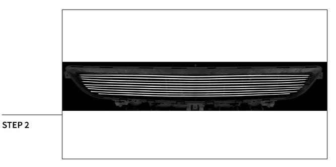
Fit the overlay to the vehicle while aligning the toggle nuts through the vehicle grille. Then, begin to tighten the Phillips bolts.
