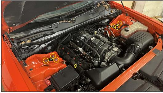
Open the vehicle hood. Remove the OEM strut covers, if equipped. Remove the engine cover (5.7L). Remove (6) 13mm upper strut nuts.
