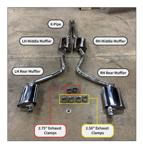
Lay out and identify all exhaust components. Once identified, remove the vehicle exhaust by removing various exhaust hangers and loosening all exhaust system clamps/flanges.
