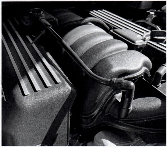
1. Locate the stock PCV line on top of the engine and remove it by pulling it off the rubber connections.
