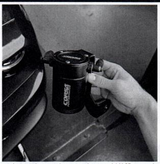
Install barbed fittings and bracket to the catch can using an 11/16" wrench and 2.5mm Hex wrench.
