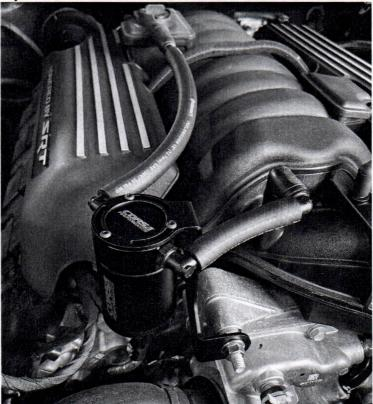
2. Use the provided nut and a 15mm socket wrench to secure the catch can bracket to the bolt extending off the front of the engine. Attach the 11" hose to the straight barbed fitting and route it to the A side of the catch can. Attach the 4" hose to the elbow barbed fitting and route it to the B side of the catch can.
