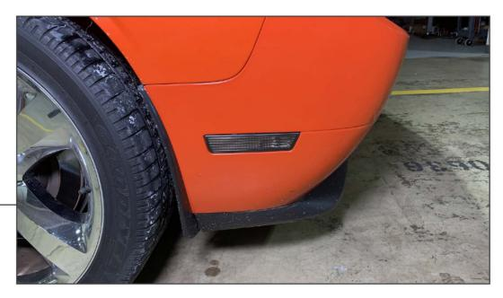
Insert (1) Amber LED light bulb into the vehicle light socket. Install the light socket into the clear side marker lamp, and press the assembly into the vehicle bumper.
