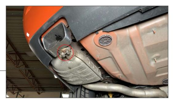
Loosen (1) 12mm clamp from the muffler and remove the exhaust tip from the muffler. Exhaust tips will be reused during installation.
