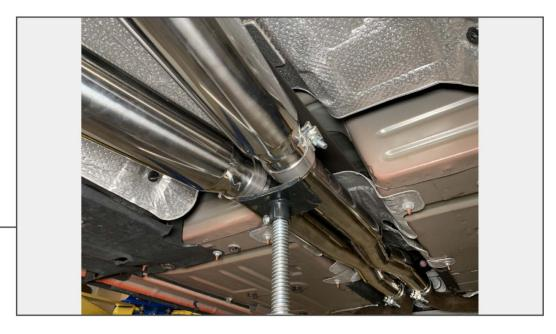
Loosely install the (2) mufflers to the X-pipe using (2) 3" exhaust clamps. Do not fully tighten at this time to allow for later adjustments.
