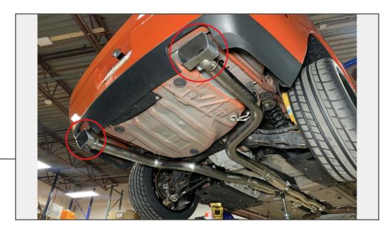
Loosely install the original exhaust tips using the provided (2) ball flange clamps. Adjust the exhaust as necessary to allow the exhaust tips to fit within the bumper cutouts. Once adjusted, tighten all hardware until secure.
