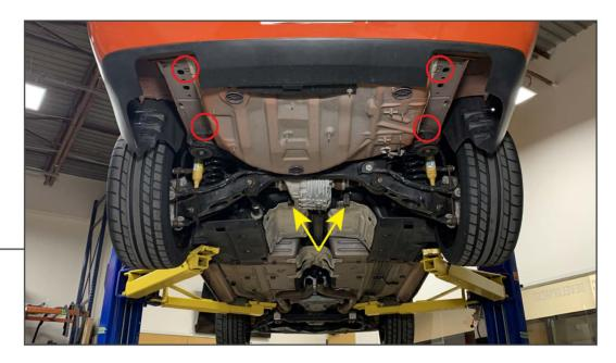
Unbolt the (2) exhaust hangers above each vehicle muffler. Disconnect (1) rubber hanger in front of each vehicle axle.
