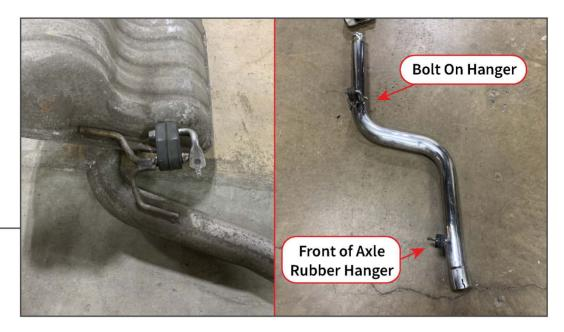
With the exhaust removed, transfer the (2) exhaust hangers to the new exhaust system.
