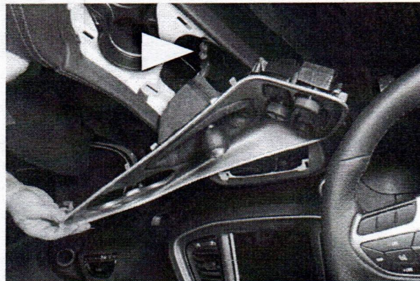
15. Remove the 2 shifter stick screws. Then remove the assembled stick, boot, and console bezel from the vehicle.
