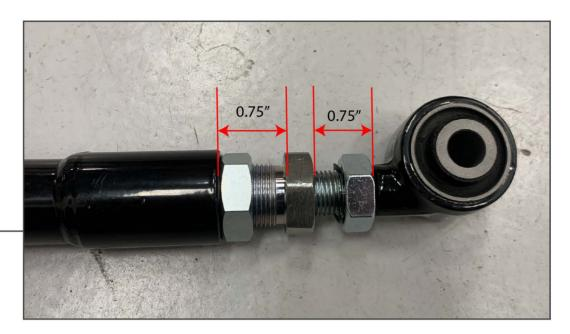
Loosen the adjustment collars to a max of 0.75". Do not exceed 0.75" of stick out.
