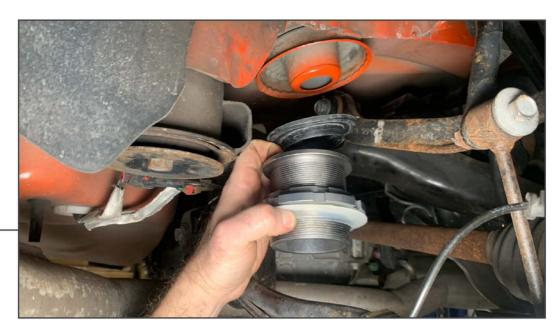
Place the adjustable spring perch in the factory location. Install the thin rubber isolator, adjustable spring perch, and nylon spring isolator. Place the lowering spring in the factory lower spring isolator.
