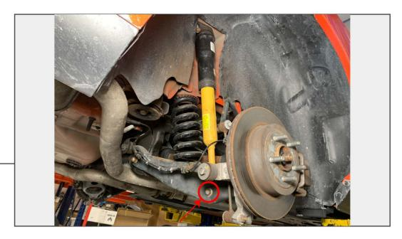
Using a 15mm wrench and 18mm socket, remove the lower should bolt. Remove the shock from the vehicle.
