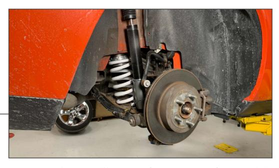
Ensure all the locking rings are tight. Torque all hardware to factory torque specifications including the lug nuts.
