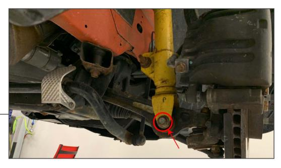
Loosen and remove the lower strut bolt.
