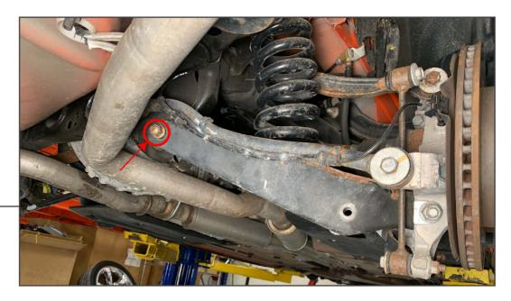
With the mufflers loose/lowered, place a jack under the lower control arm to support the control arm/spring tension. Using a 15mm wrench and 18mm socket, remove the inner lower control arm nut and bolt. Slowly lower the jack/control arm to relieve the tension from the spring, then remove the spring from the vehicle.
