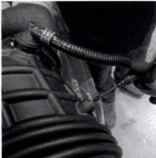
11. Remove the air temperature sensor from the factory air duct.
