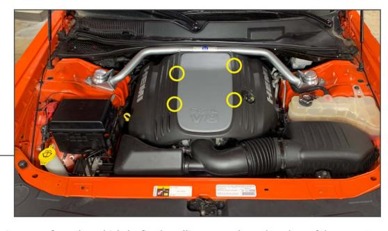
Remove the engine cover from the vehicle by firmly pulling upwards on the edges of the cover to dislodge the (4) pins from the grommets.
