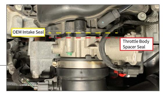
Install the throttle body spacer in between the intake manifold and the throttle body. Ensure the OEM intake manifold seal remains in place. Use the provided throttle body seal to meet the throttle body spacer to the throttle body.
