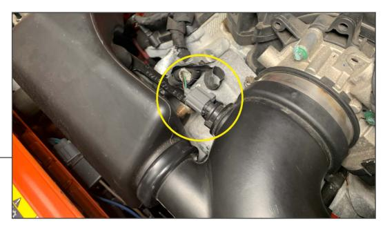
Unplug the electrical harness from the IAT sensor by depressing the plastic tab on the connector.
