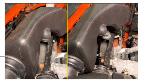
Firmly lift upwards on the intake tube resonator to dislodge the tube from the mounting bracket grommet. Lift and remove the intake tube from the vehicle.
