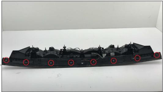
Using a Phillips head screw driver, remove the screws securing the factory tail light trim to the
