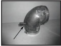
Step 10 Install the supplied grommet into the 90°coupler then install IAT sensor into the grommet.
