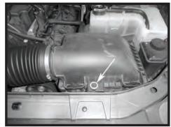
Step 4 Remove the screw holding the factory air box in place.
