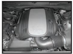
Step 2 Remove the engine cover.
