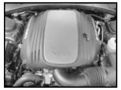
Step 2 Remove the engine cover.
