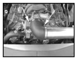
Step 12 Install the 90° coupler onto the intake tube. Once on the tube, place the other end of the coupler over the throttle body. Fully tighten the clamps.
