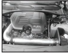
Step 20 Reinstall the engine cover. Make sure that all clamps and hardware are fully tightened. Reconnect the battery cable, start the vehicle and let it warm up. Shut off and inspect the installation once more for any loose clamps, wires, or hardware. Test drive & enjoy! Your installation is now complete. Periodically check all clamps and brackets.
