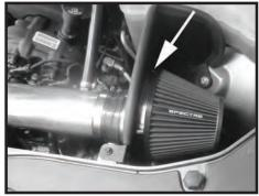
Step 19 Install the filter on the velocity stack adapter and fasten it securely. If required rotate the velocity adapter so the filter will fit without any fitment issues.
