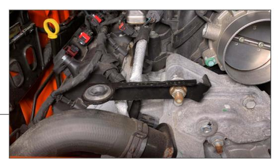
Remove (1) 16mm nut from the retaining bracket to remove the bracket from the vehicle.
