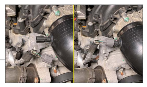
Plug the electrical harness into the IAT sensor. Ensure the connector clicks into place for proper connection.
