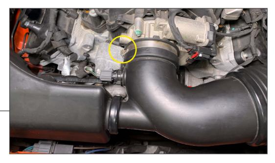
Using a 8mm socket, loosen the (1) hose clamp securing the intake tube to the throttle body.
