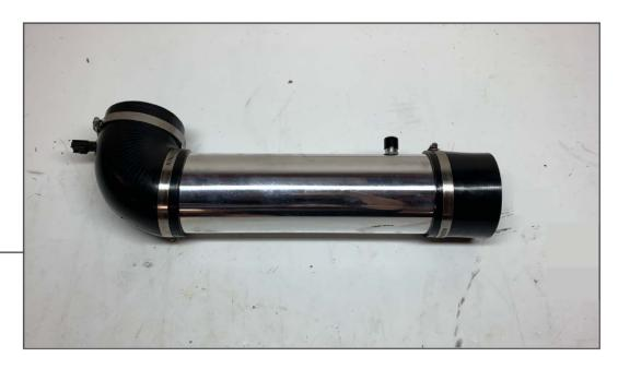
Assemble the intake tube using (4) 4" hose clamp, (1) 90 degree coupler, and (1) straight coupler.
