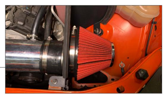
Install the air filter to the air filter adapter using (1) 6" hose clamp. Tighten until secure.
