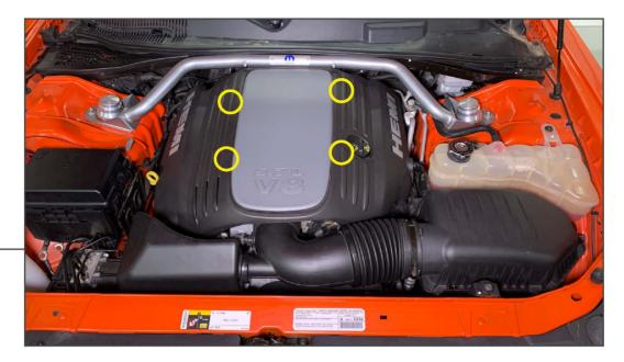
Remove the engine cover by firmly lifting along the sides of the cover to dislodge the (4) mounting pins from the cover grommets.
