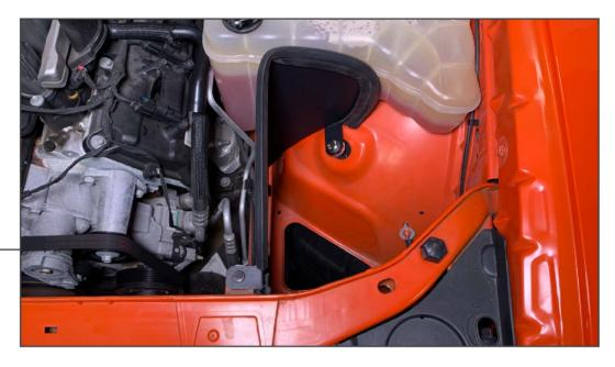
Install the heat shield into the vehicle using (1) 3/8" bolt, (1) 3/8" flat washer into the previously installed threaded insert. Install the front of the heat shield using the original 8mm bolt.
