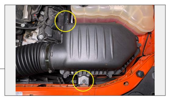
Remove (1) 8mm bolt from the front of the air box. Remove the PCV hose from the air box.
