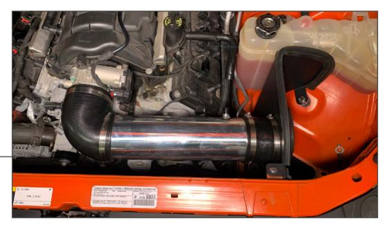
Install the intake tube to the throttle body by placing the coupler over the throttle body. Loosely clamp in place.
