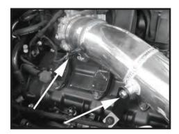
Step 17 Reconnect the IAT sensor connector. Fasten the bracket to the intake tube with the supplied hardware.
