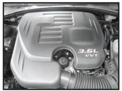
Step 2 Remove the engine cover.
