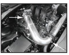
Step 16 Install the second intake tube into the throttle body coupler first then into the flex coupler. Once in desired position fasten securely in place.
