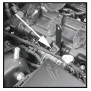
Step 12 Install the bracket onto the mounting stud as shown.
